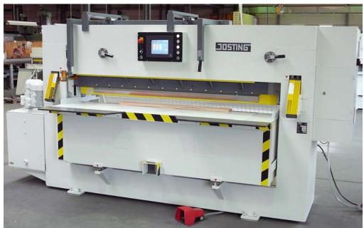
The machine cuts veneer packs exactly parallel and straight on two sides with top and bottom knife.
