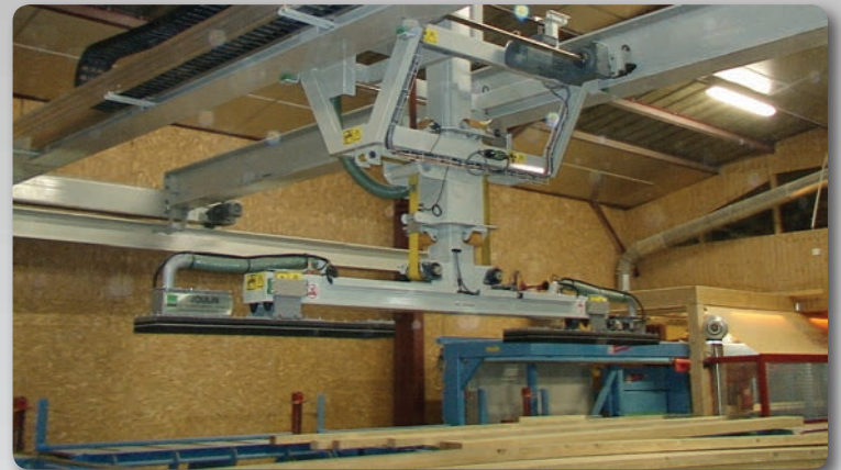
Example of stacker/destacker to load/unload a CNC
