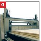
When the pressing process is finished the elements are pushed onto the outlet table. The clamping carriage of this table passes over the elements and pushes it/them on for further processing.
