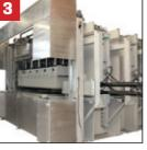
The fully automatic press brings a lamination pressure of 10 kg/ cm<sup>2</sup> from the top plane. This pressure is generated by sturdy hydraulic cylinders. All cylinders can be disconnected individually allowing the pressure pattern to fit the shape of the element, e.g. over door and window openings.
