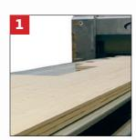
Before the CLT element enters the press line it is shaped and laid up on a plastic board in the requested number of layers. Glue is applied between each laver.
