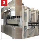
The fully automatic press brings a lamination pressure of 10 kg/ cm<sup>2</sup> (150 PSI) from the top plane. This pressure is generated by sturdy hydraulic cylinders. All cylinders can be disconnected individually allowing the pressure pattern to fit the shape of the element, e.g. over door and window openings.
