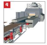
The completed product charge is fed into the high frequency press where it is pressed from the side and the top and the high frequency energy is added for a rapid curing.
