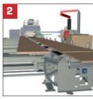
When manufacturing CLT elements, the glue is applied to the side of the longitudinal lamellas. The lamellas are cross conveyed to a temporary collection unit, where they are joined together and lifted onto a belt conveyor for adding more layers.
