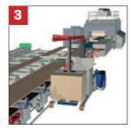
A special designed glue trolley applies glue on top of the longitudinal lamellas and then the cross lamellas are positioned by means of a vacuum lift installed on the glue trolley.
