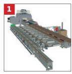
When manufacturing glulam beams, the glue is applied from above. The glued lamellas are cross conveyed one by one, turned 90°, joined and fixated in a charge. Following this, the charge is loaded onto a belt conveyor which feeds it into the press.
