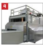
In order to optimize the production line further to an order-based production, the press can be manufactured with semi-automatic setting of the press height enabling different products to be pressed in rapid succession, and with side pressure widths from 1280 mm and down to 240 mm, so that single and few beams can be produced by themselves according to order. Flexibility is the keyword.
