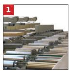
The line is fed by a high speed dual roller conveyor, allowing the lamellas to be conveyed to the lay-up system at a quick pace. The lamellas are cross conveyed in two steps, in order to prevent collision during transport.
