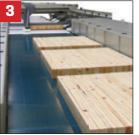
The inlet conveyor in front of the HF/RF-press is equipped with side supports to prevent the lamellas (short lamellas especially) from overturning during transport into the press.
