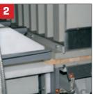
The glued lamellas are fed into the fully automatic press which consists of two parts: a high frequency unit in front and a hot
