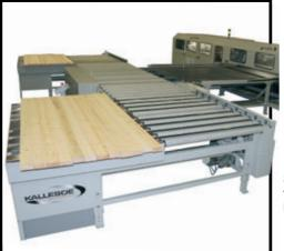
Vacuum gantry for quick and efficient destaking from the line
