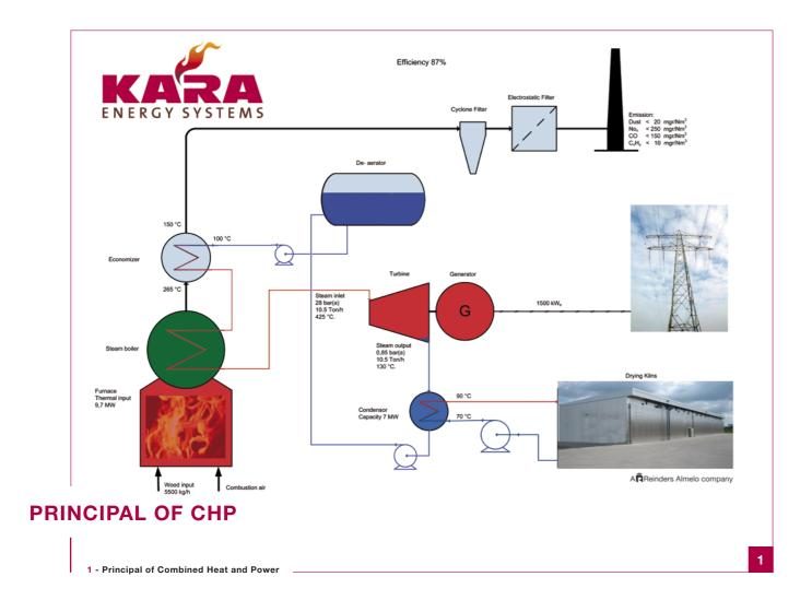
where the steam is expanded, and thereby producing mechanical energy. The mechanical energy can be transformed into electricity with a generator. The steam coming out of the turbine is lower in pressure and temperature than the entrance conditions. The pressure drop drives the turbine. The low pressure steam is condensed to produce warm water. The condensate is pumped back to the steam boiler.
