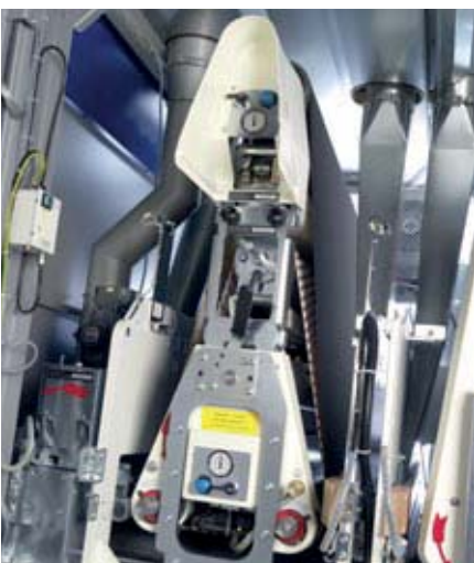
Longitudinal sanding unit (with pressure segment belt)
