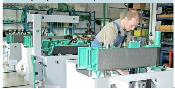
The ultimate in edge sanding is the KÜNDIG Uniq. A heavy cast iron working table is provided on one side for solid wood sanding, along with a similar one on the other side for veneer sanding. The height adjustment and the tilting of the abrasive belt are motorized and no adjustment of the working tables is required. Ingenious and therefore patented worldwide.
