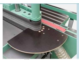
Semi round table for sanding curved pieces against the rubber covered driving roller
