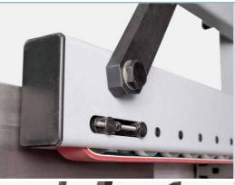
Instead of pressure rollers, the upper feed belt can facilitate the sanding of smaller components
