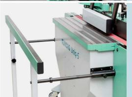
Easy handling of large panels thanks to the telescopic support rail
