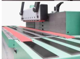
For larger workpieces an additional lower feed belt can be provided
