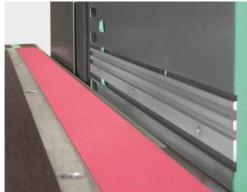
The grooved inlet platen allows the sanding of edges with overlapping veneers
