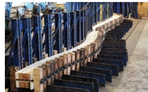
CURVED LAMINATED BEAM IN PRESSING BED
