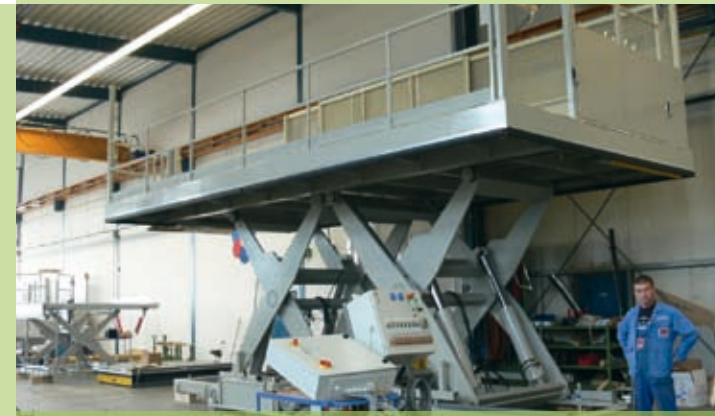
LAWECO LOADING LIFT TABLE with hydraulic loading bridge, railings and doors
