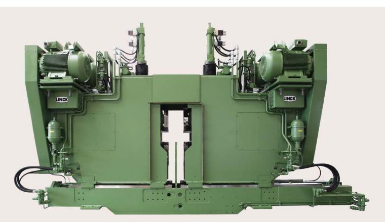
The two VPM machine halves are supported on linear guides. The generous length of the linear guides offers comfortable space for changing tools when the machine is in tool changing position.
