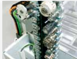
Chain-type tool magazine with 16 or 32 places
