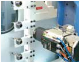
Linear-type magazine with 6 tool places
