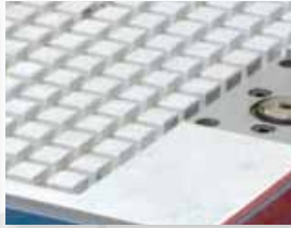
Aluminium grid table with milled slots
