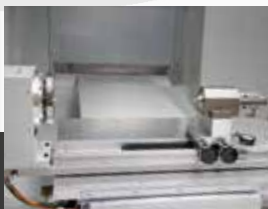
NC rotational axis on table
