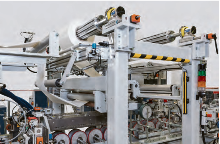
Double foil unrolling with automatic transport connection and infrared heating.
