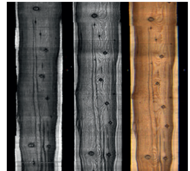
Goldeneye 900 features Multi-Sensor cameras and sensors for laser scattering, laser 3D triangulation and color analysis
