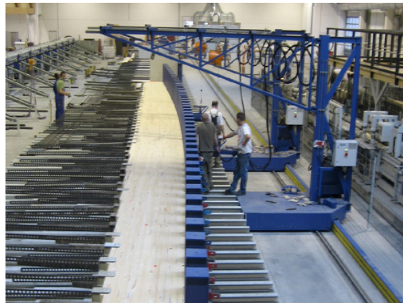
Automatically adjustable pressing bed with movable carriage and hydraulic tightening device
