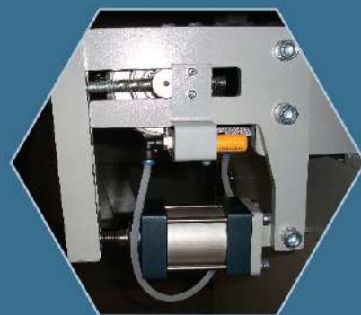
Automatic device for feed belt tracking 輸送帶自動導正裝置
