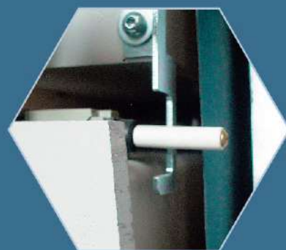
Security switch by ceramic bars 砂帶安全開關
