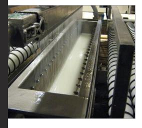
Today I use a roller spreader, what advantages has the separate system from Mixon? ■ First of all the adhesive will be applied separate, which means no mixed glues and no more end of Open Times and no more cleaning.
