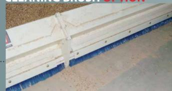
The brushes, combined with a good quality concrete floor, reduce the remaining layer of product to an insignificant quantity.
