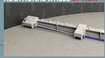
Must be installed as soon as the diameter of the silo exceeds 22 metres and mechanically connected to the main wheel, it optimises the emptying time.
