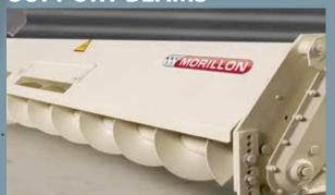
They ensure perfect rigidity of the MORILLON auger and an optimum alignment over its entire length. A system of openings on the front panel controls the product flow on the auger itself.
