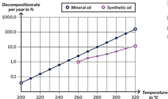
Light-ends evaporate and ignite even at low temperatures and may endanger the operational safety.
