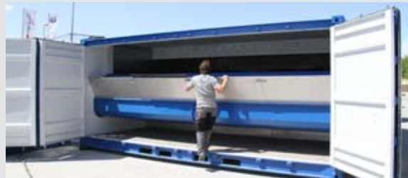
QX for large scale drying, belt width 5.450 mm
