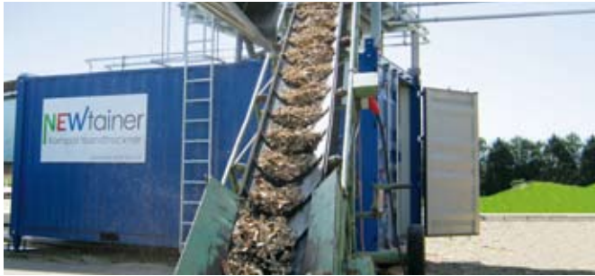
WT 0.5 in use in wood-chip drying
