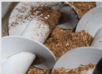
NEWtainer® QX Feeding-system with double screw.
