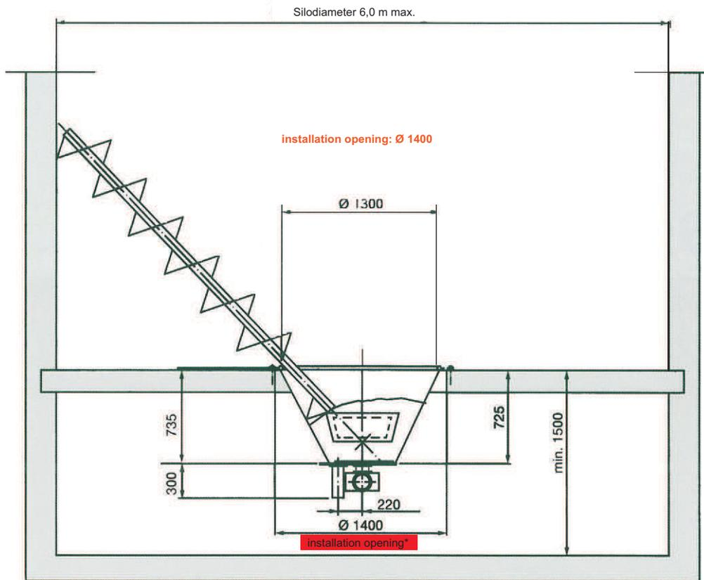
\* The installation opening must be made by the customer.
