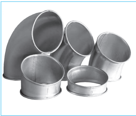
QFS Pressed Bends (long radius) R=1,5 x diameter to centreline
