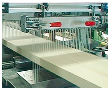
Separate application of resin and hardener to glulam lamellas
