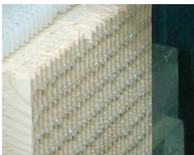
Glue threads on the finger peaks, crosswise to the profile
