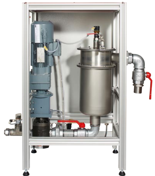
Dosing unit KONTITOP with gear pump for continuous processes
