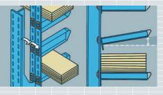
The patented boltless slot-in arm assembly enables the cantilever to move freely on impact, protecting products and racking from damage. The height-adjustable arm can be easily adapted to any goods stored.
