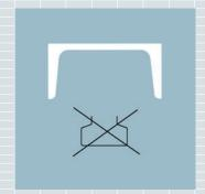
Hot-rolled steel profiles instead of thin wall sheet metal.
