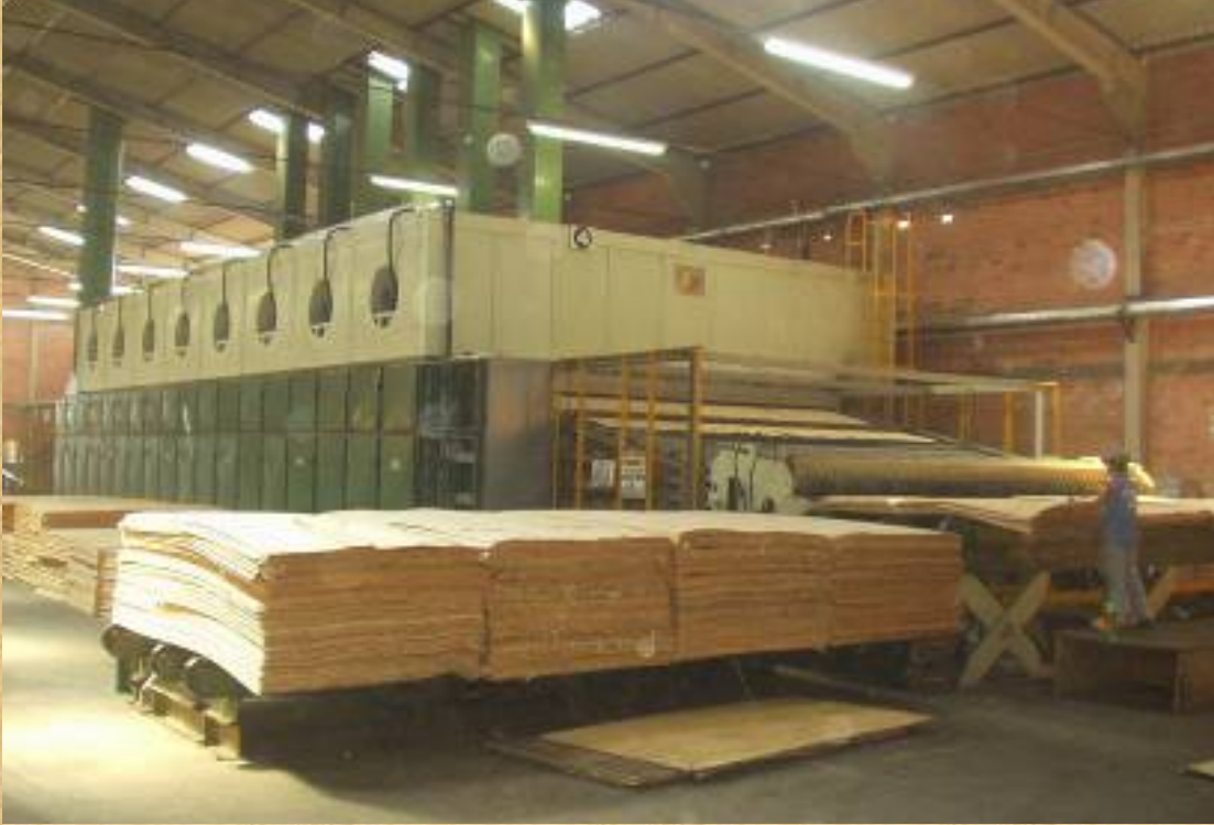
Semi automatic feeding system with cross chain feeder, heavy duty lift table with cross chain and indexing tipples
