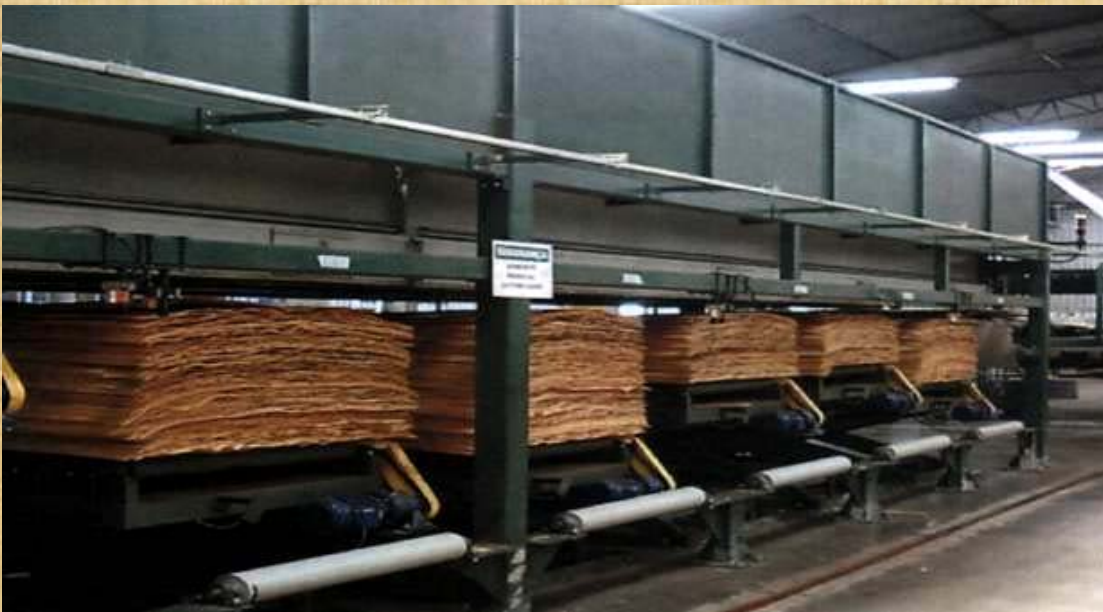
Automatic vacuum stackers with manual or Automatic veneer grading.
