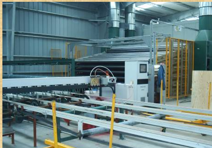
Dryer out feed with sequential unloader, cross transfer, moisture detector and dry chain conveyor
