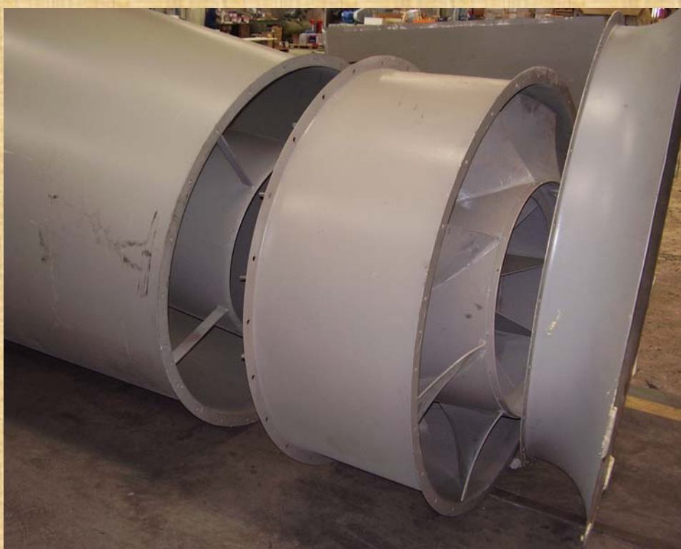
Carbon steel axial fan to high flow with highest air temperature
