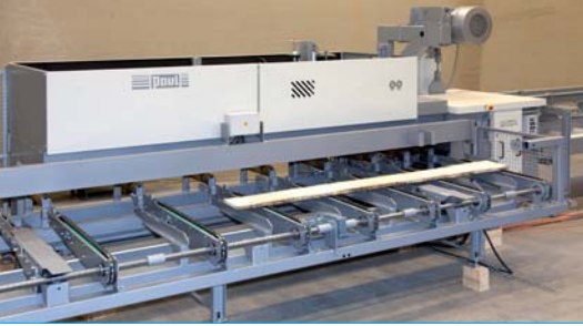
AB920 fully automatic infeed system combined with a KME3-1012 with overhead motor
