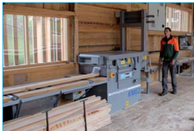
KME2-750 Circular Edger, manually loaded, operating in a sawmill
