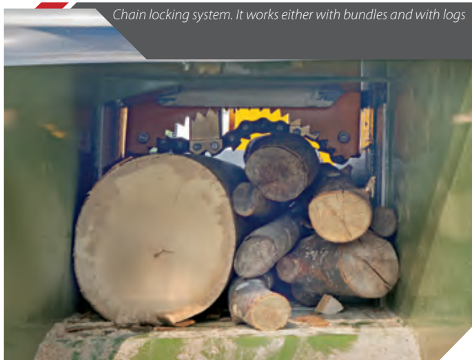
Chain locking system. It works either with bundles and with logs
