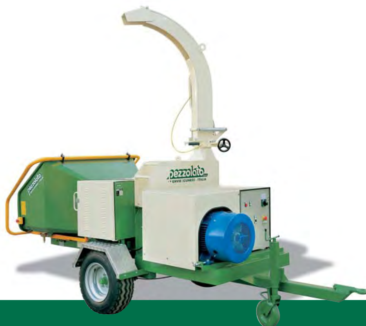
PZ 250 G at work, mounted on trailer for low speed transport. This version has a 3-point hitch and support feet.
