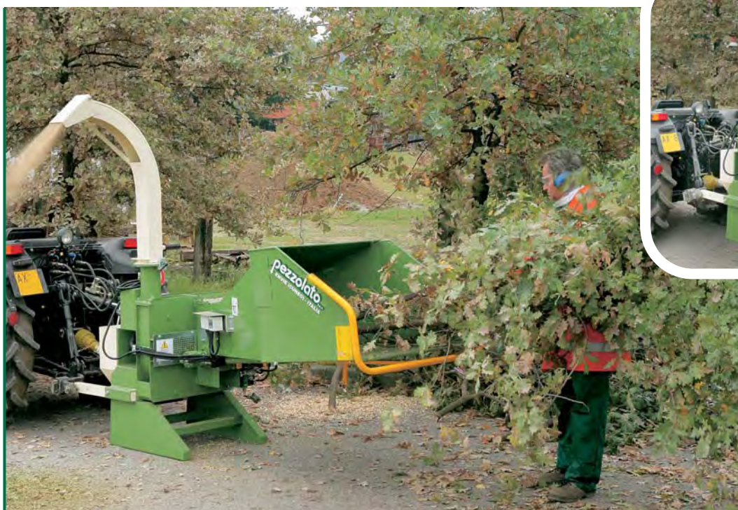
The PZ 110 G version at work. It is driven by PTO and equipped with the attachment to the 3-point hitch of the tractor. In the detail, the machine is compacted into the journey position.
