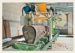
• The machine's head has been sized to allow cutting **logs** with diameter up to 1200 mm.
