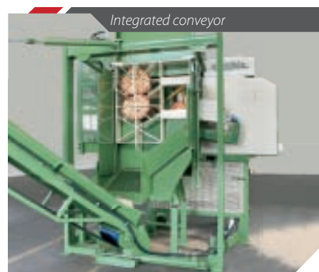
C-shaped log separating system
