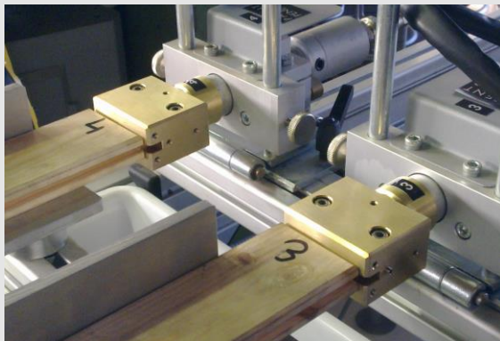
(C) Brass nozzle for coped profiles for 5 parts cabinet doors
