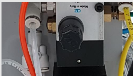
Pneumatic timer Time adjustment of the glue gun which controls the glue dispensing time
