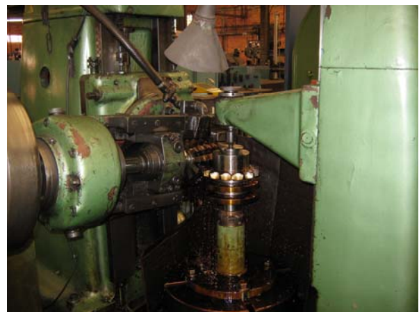
Straight/helical gear cutter, 710mm maximum diameter
