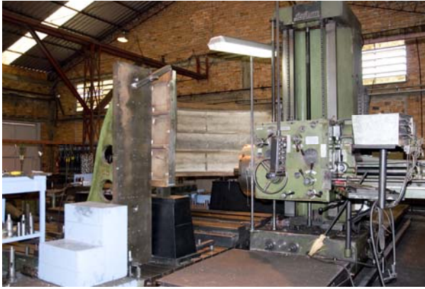
- Defun Floor type and table milling machine – 10ton working piece maximum weight – X=6.000, Y=1.500, Z=4.000mm
