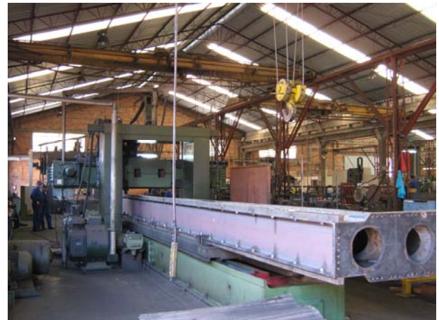
Planing/milling machine – Machining operation on 10m long
