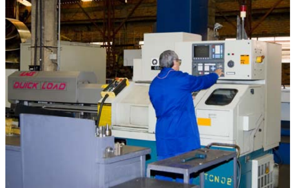
Romi Cosmos 10u CNC Turning Lathe with automatic loader
