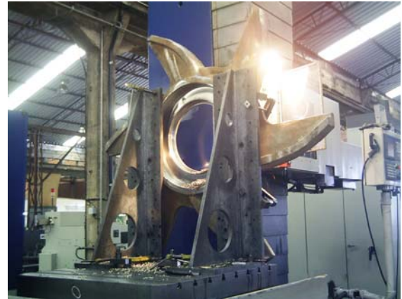
Machining operation on stainless steel rotor
