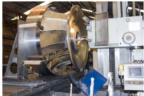
Machining operation on hydroelectric power plant rotor
