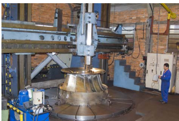
Vertical Lathe, 4.270mm maximum diameter – Machining operation on hydraulic turbine rotor
