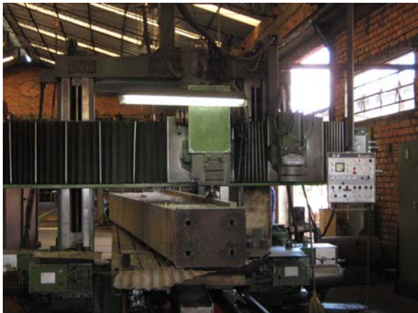
Milling machine maximum 6.000 x 2.050 wide x 1.4 m high parts
