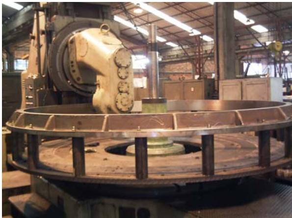
Inside/Outside straight/helical gear cutter, 3.300mm maximum diameter. Machining operation on casting iron gear with inside teeth
