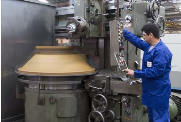
Vertical lathe, 1.200 mm maximum diameter
