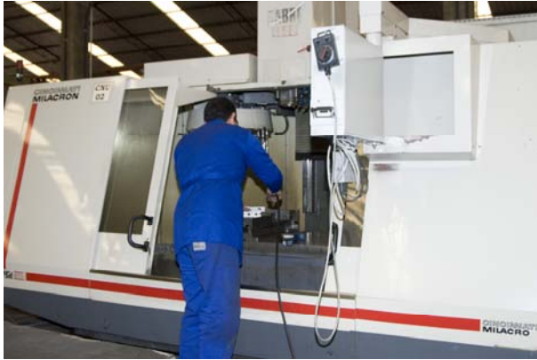
Cincinnati CNC Machining Center – X=1.524, Y=762 e Z=820
