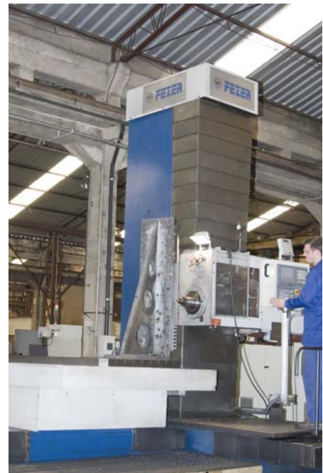
FEZER 763 Milling Machine – 6ton working piece maximum weight – X=1.990, Y=2.000 e Z=2.000
