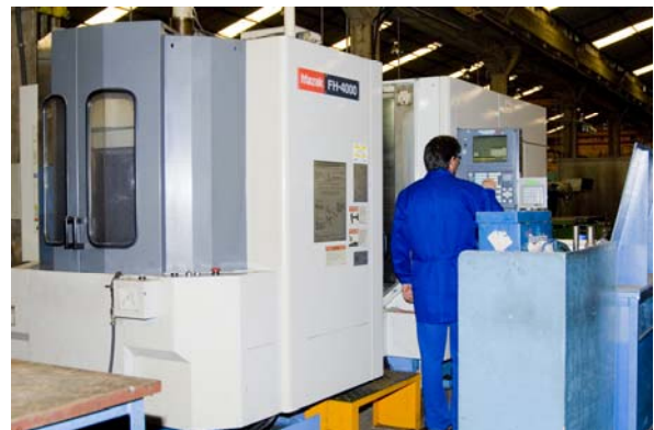
Mazak FH 400 CNC Machining Center, X;Y;Z de 560 x 510 x 630 mm
