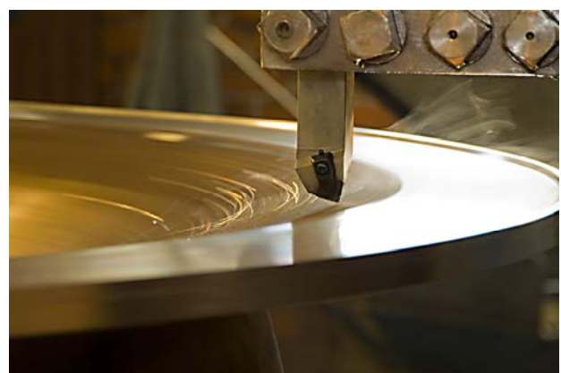
Vertical Lathe, 4.270mm maximum diameter – Machining operation on hydraulic turbine rotor
