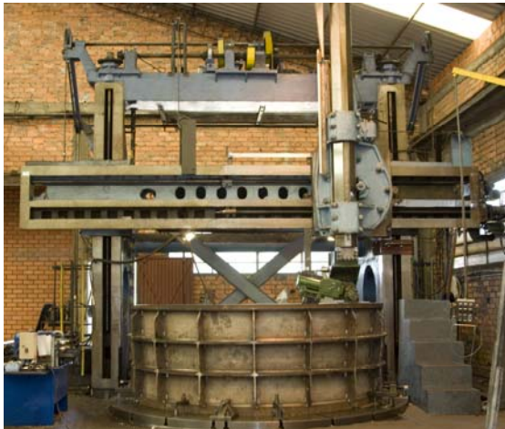
Vertical Lathe, 4.270mm maximum diameter. Machining operation on hydraulic turbine stainless steel carcass
