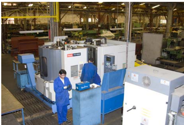
Mazak FH 400 CNC Machining Center, X;Y;Z de 560 x 510 x 630 mm
