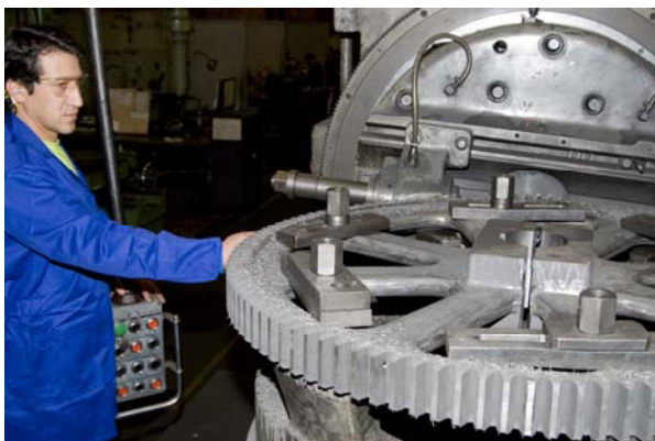
Inside/Outside straight/helical gear cutter, 3.300mm maximum diameter. Machining operation on casting iron gear with outside teeth
