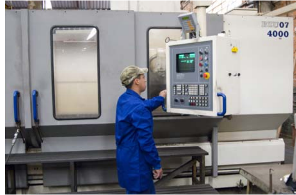
Heller CNC Machining Center – X=4.000, Y=500 e Z=560
