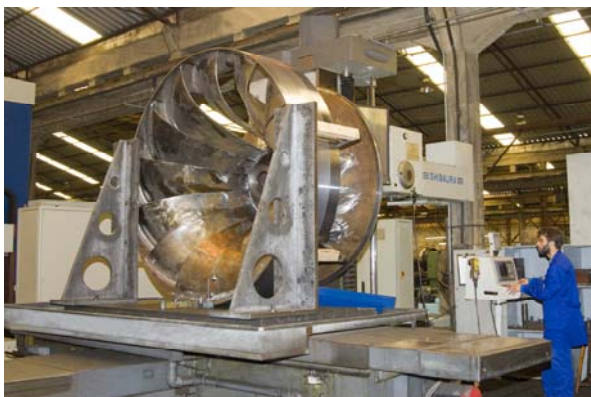
Shibaura Milling Machine – 6ton working piece maximum weight – X=2.300, Y=1.400 e Z=1.400
