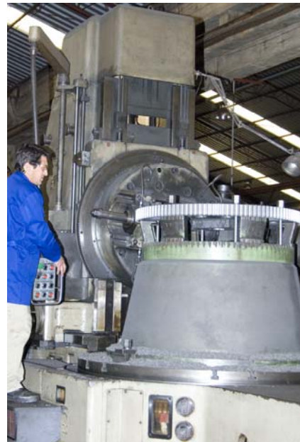
Inside/Outside straight/helical gear cutter, 3.300mm maximum diameter. Machining operation on casting iron gear with outside teeth
