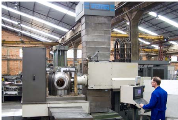
Wotan Cutmax2 Milling machine - 4ton working piece maximum weight – X=1.800, Y=1.700 e Z=1.500
