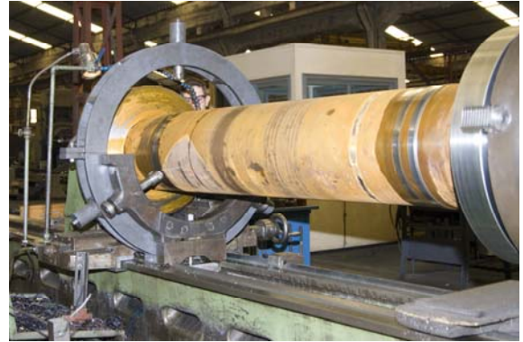
Conventional turning lathe – 800 mm diameter x 5.000mm
