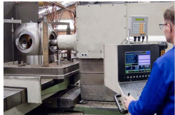
Machining operation on rotor valve, casting steel
