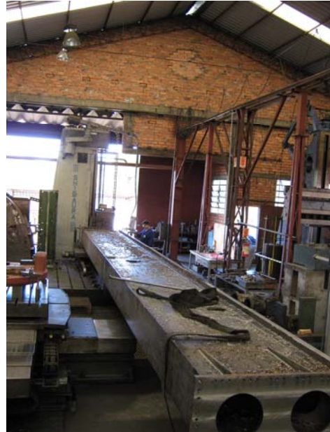
- Shibaura floor type and table milling machine – Machining operation on elevation column
