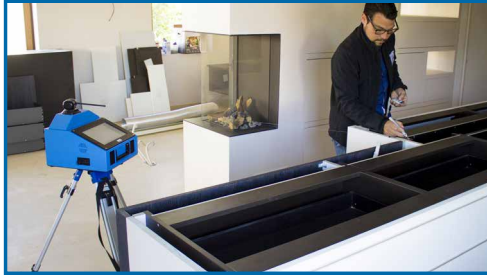
Proliner CT Template countertops and backsplashes on-site
