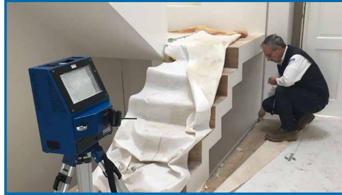
Proliner CT Create digital templates for flat glass constructions
