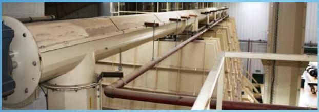
PST Shaftless Spiral Conveyors are widely used in pellet plants all over the world. We transport everything from incoming chips, wet and dry sawdust to wood powder. A common need for pellet production is to lift materials to the different levels of the factory, such as from incoming materials storage to the dryer, from the dryer to storage bins, from storage bins to the hammer mill, the hammer mill to the pellet press and so on...
