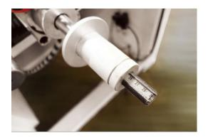
6. Pressure cylinder : adjust material thickness and vertical and horizontal distance according to sheet size by the adjustable handle , the distance of each row is 10 mm
