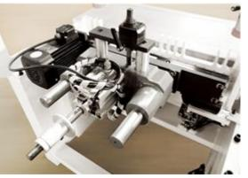
5. Drilling components have drilling depth adjusting device, scale values on ruler's flat end show drilling depth.
