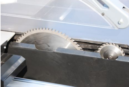
3.Main saw blade and groove saw blade: angle of inclination is shown by the precision goniometer.
