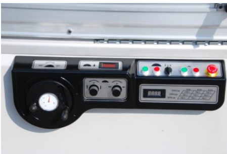
5. Control Panel: angle of inclination is shown by the precision goniometer.
