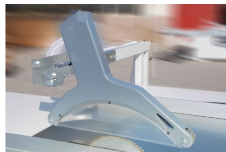
6.Suction hood: equipped with European style suction hood makes the machine with a reasonable structure and strong power for suction.
