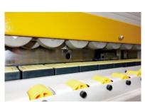
(b). Electric type pressure beam lifting system is the optional configuration. But it as the standard configuration for the machine with pre-milling function. The rise and fall of the pressure beam can be fast started on the operation screen, lifting height can be showed on a separate position indicator.
