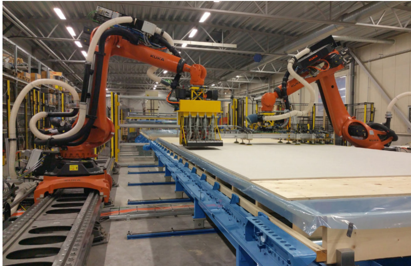
Robot 1 equipped with screwing tools initiating screwing process, robot 2 holding gypsum sheet in place ensuring accurate placement during part of screwing process
