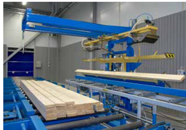
Timber picker with additional roller conveyor system
