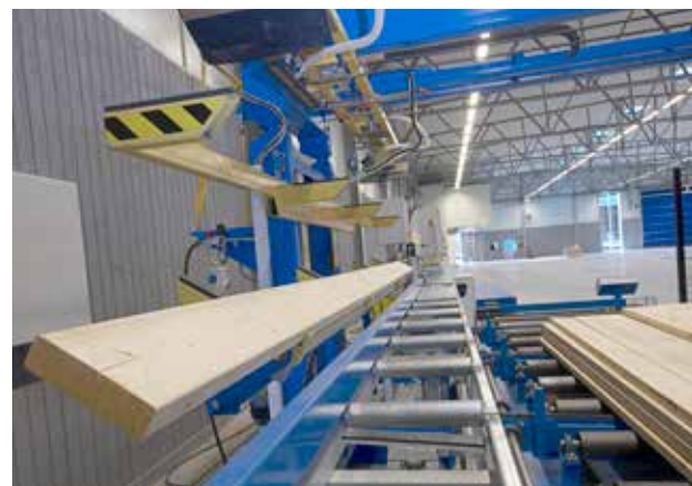
Board is ready to be slid or flipped down to the infeed bench.
