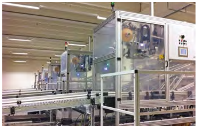
High-performance servo labeling device
