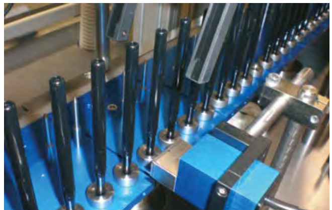
Precise application of oil on plastic parts
