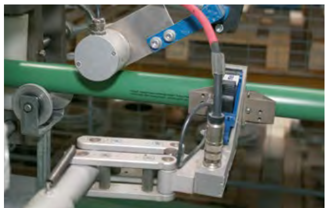
Contact-free coding and marking of extruded pipes
