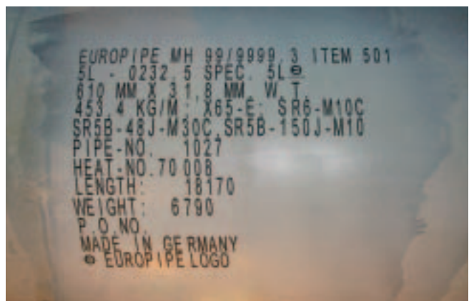
Color mirror engraving in steel pipe production
