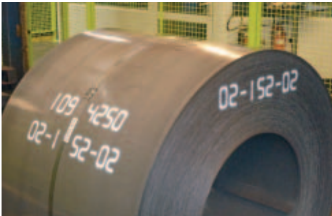
Marking of steel coils
