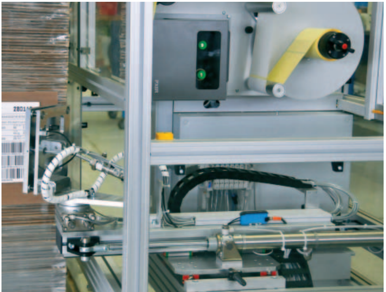
Pallet labeling in conformity with CCG/GS, 1 stop for 2 at right angles
