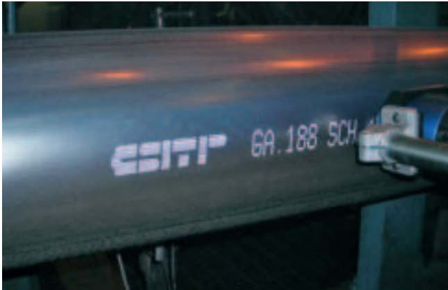
Coding of pipes (steel, plastic etc.)
