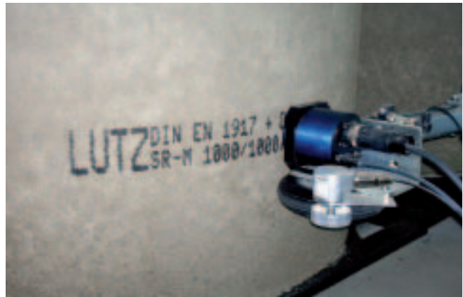
Marking of concrete pipes
