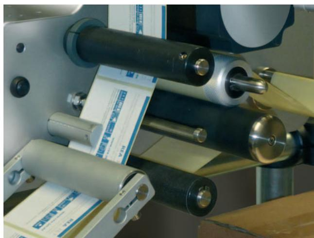
Dispensing widths from 100 mm to 200 mm at dispensing speeds of up to 120 m/min are possible with the REA JET ES label dispenser
