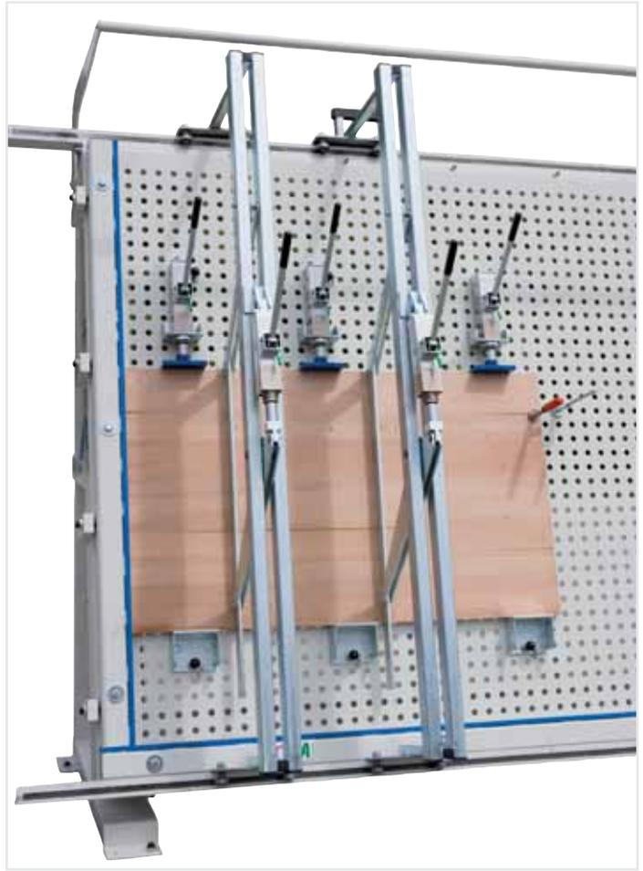
The range of accessory items is diversified. Rotating and non rotating pressure cylinders are available options in both hydraulic and pneumatic. They are complemented by various single abutments.
