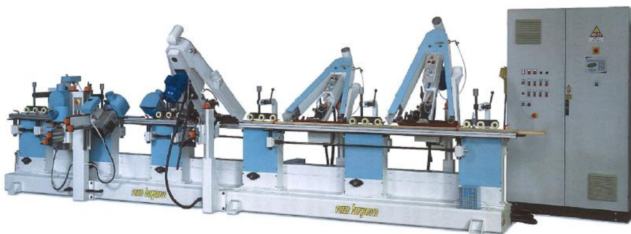
Renzo Borgonovo Srl Sanding machine with a mix of Scotch Brite and Sanding Belt units
