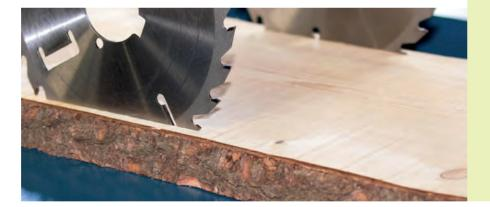
High precision: The plank remains stationary on the table, while the sawhead travels back and forth. Two pressure rollers in front and behind of the saw blades hold the wood in place with downward pressure during the cutting process. This new manufacturing process is unique to the market and guarantees an exact, parallel and straight cut.
