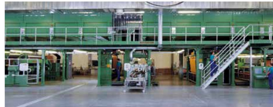
Lacquering machine with two units and double-layer coating
