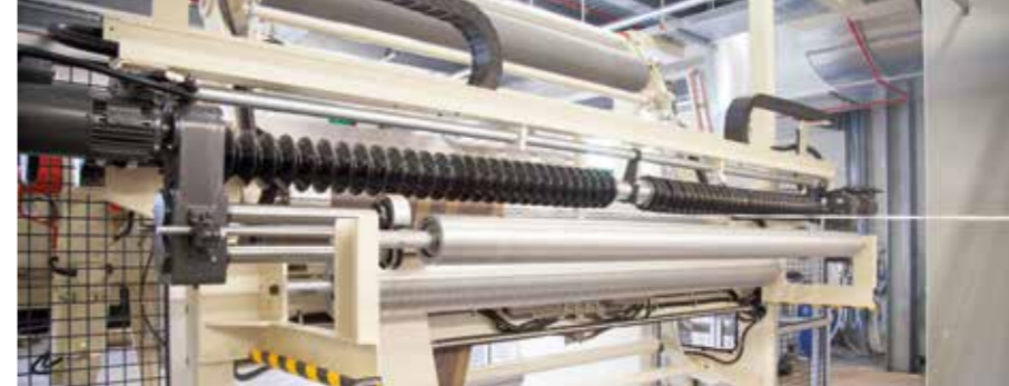
Winding technology with non-stop changing of rollers
