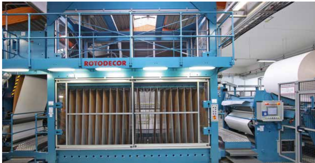
Web splicing system for butt-joint and festoon section
