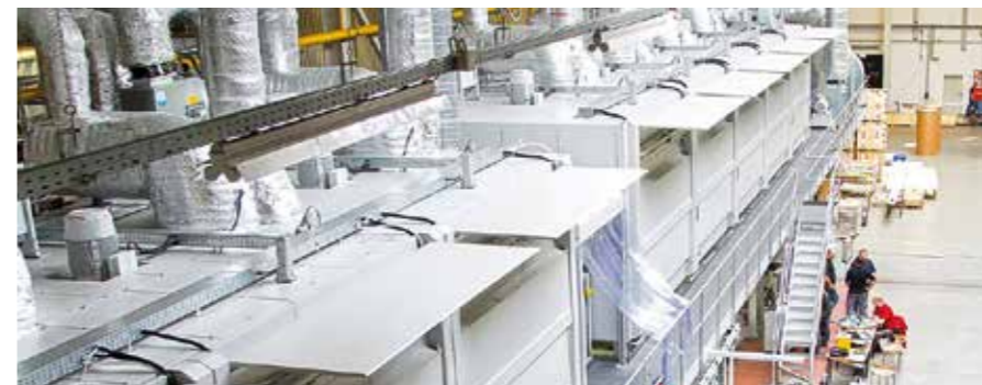
Dual station lacquering machine for double layer coating
