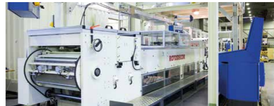
Stacker with stack turning device
